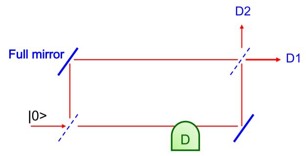
Any device able to detect photon (non-destructively)
